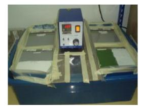
Accelerate test that each specimens immerse in the water 3/4 depth of specimen thickness. Water temperature keep 35 °C, ambient temperature is 20°C, 5 weeks.
