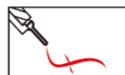
3. Press the ceramic tile grout glue gun, squeeze out about 30-50cm glue to avoid uneven mixture
